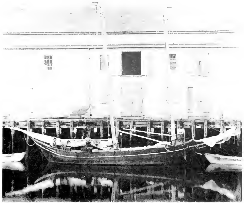
NEW ENGLAND PINKY from Friendship, Maine, showing a typical vessel of the type. (Smithsonian photo 34911-g.)
